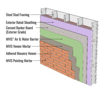
Framed wall with cement backer board substrate
