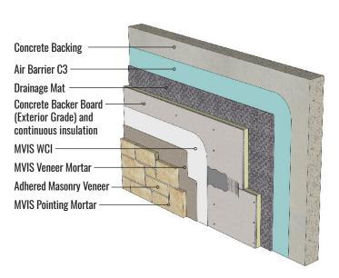
Framed wall with drainage mat, and continuous insulation cement backer board
