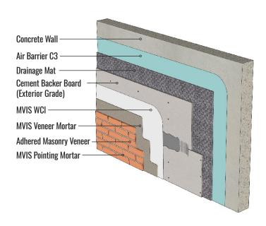
Concrete wall with drainage mat and cement backer board
